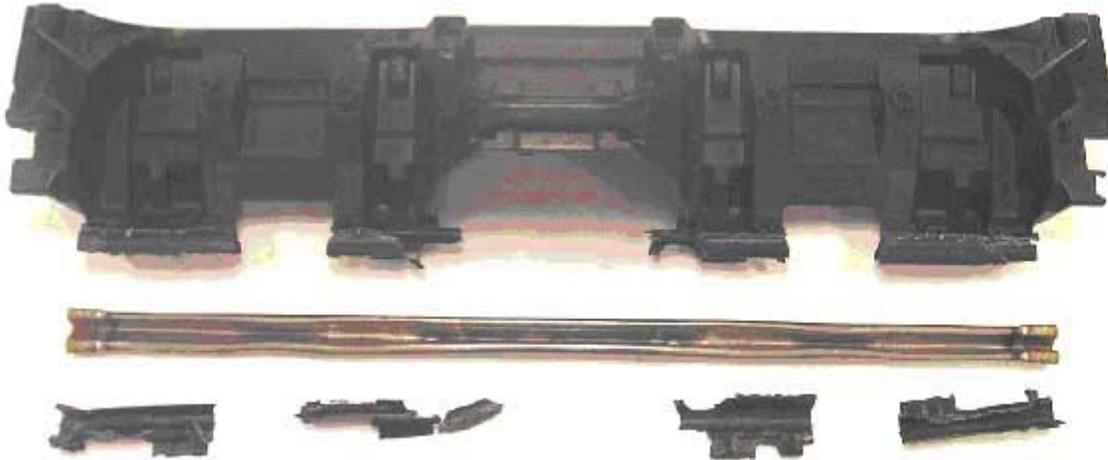
*Figure 7: The hybrid steel/composite IP carrier can easily be disassembled and recycled at end of vehicle life. By using a standard hydraulic shearing machine, the beam can cleanly be removed from the rest of the composite carrier.*
