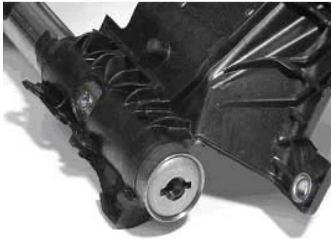
*Figure 13: Owing to 2 technology breakthroughs – a special grade of GMT material and a patented process to prevent crushing of the steel tube during molding – the CCB is fully encapsulated at key junction points on the lower IP carrier.*
