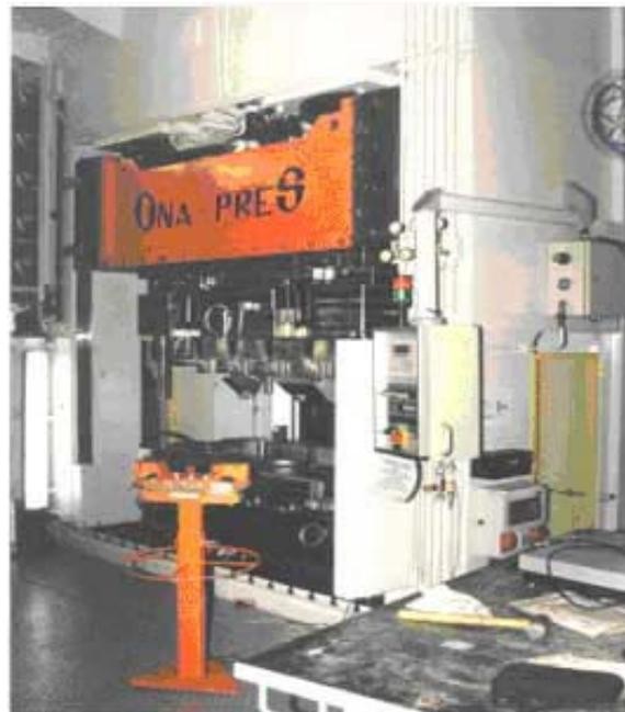
Figure 9: Vertical compression molding press for production of the IP carrier ..
