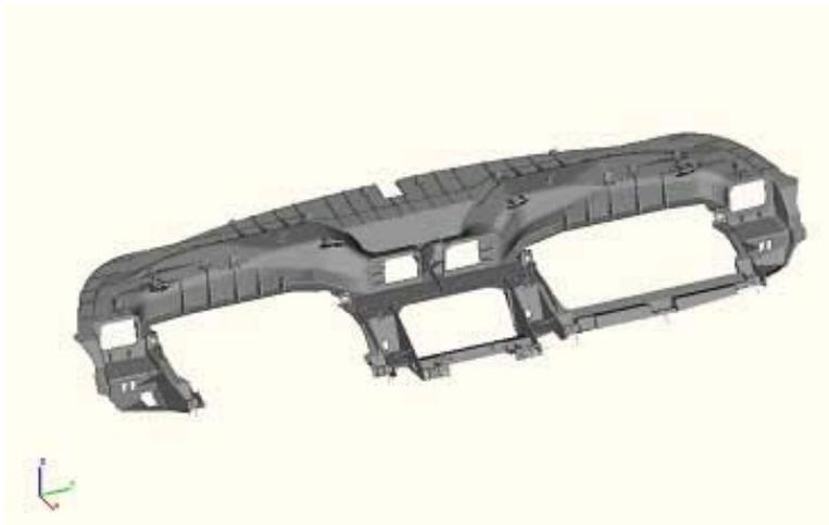
*Figure 4: The upper IP frame is injection molded from LFT polypropylene with 40% long-glass fiber reinforcement. The lower IP carrier is subsequently vibration welded to the upper IP frame.*
