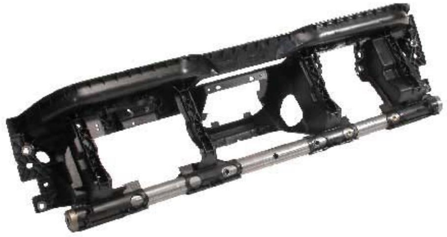
Figures 14 & 15: It was very important to maintain strong knitlines at junction points between the CCB and the GMT carrier. This was accomplished by careful control of process parameters, particularly pressure.
